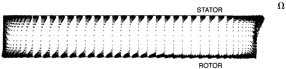
Figure 17 Radial flow in a rotor–stator system without throughflow
